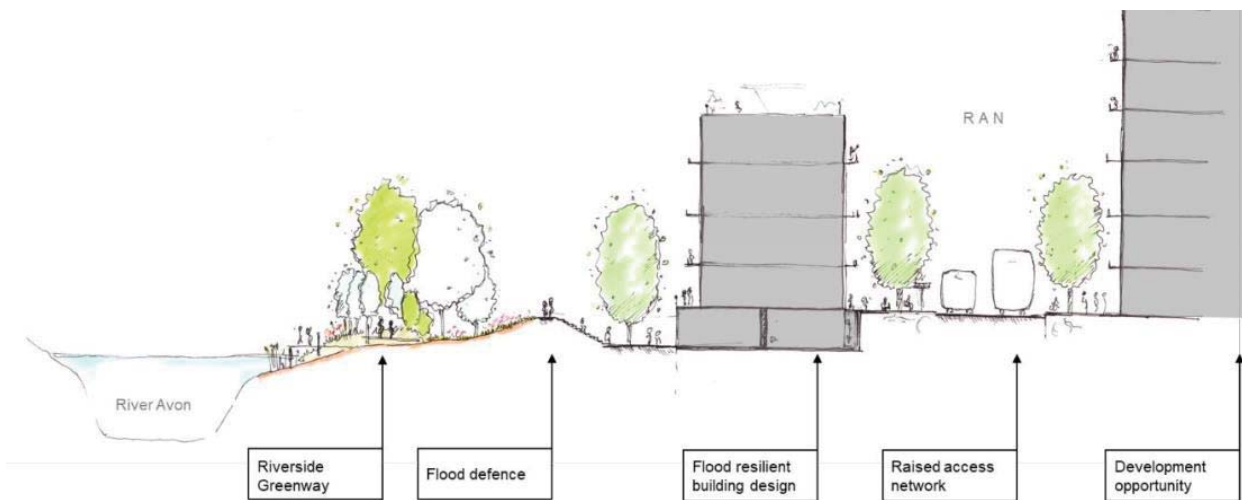
Figure 24: Example of how flood defences can be incorporated into BTQ development 18
